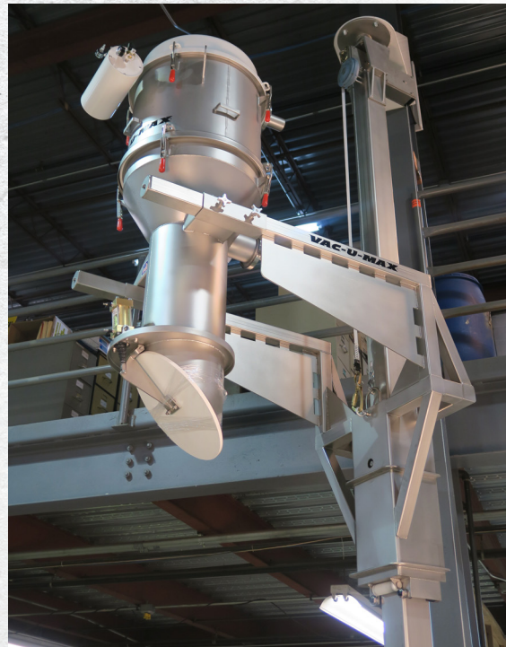
Floor-mounted Column-Lift Vacuum Receivers are ideal for applications requiring from-floor conveying up to 25 ft above processing or packaging equipment
