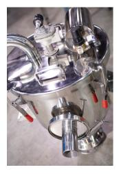
Peak performance comes from fine tuning and knowing which components will move the material most gently, reducing wear and degradation. All equipment must complement each other. Vacuum receivers must be able to handle the airflow provided by the vacuum source and balancing the air-to-cloth ratio of filters must occur, so filters don't shred or blind.
