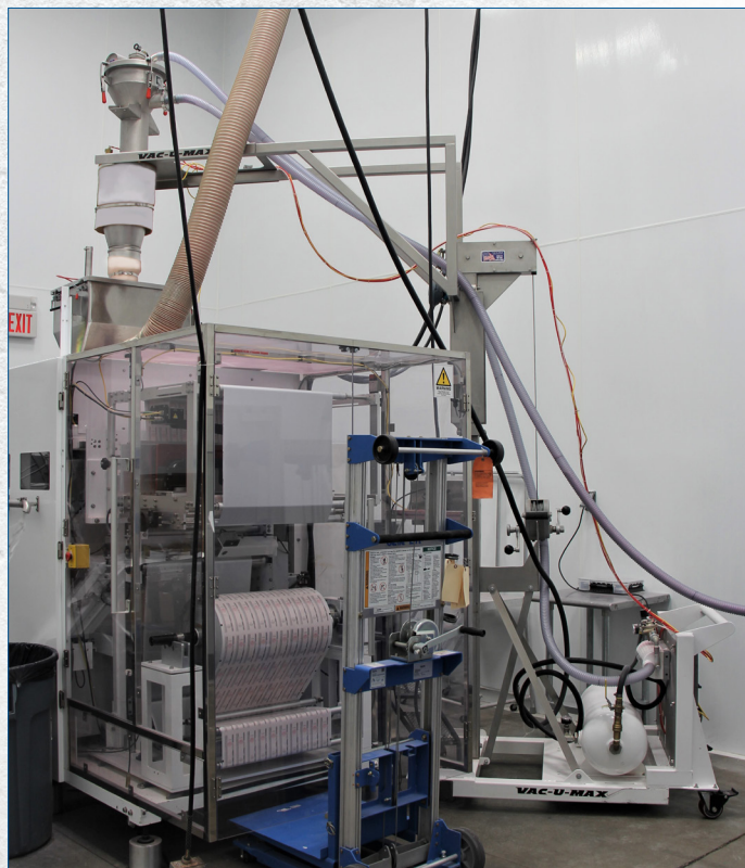
Mobile Vacuum Conveying System provides continuous supply of material from containers at floor level up and over to refill stick packaging machine.
