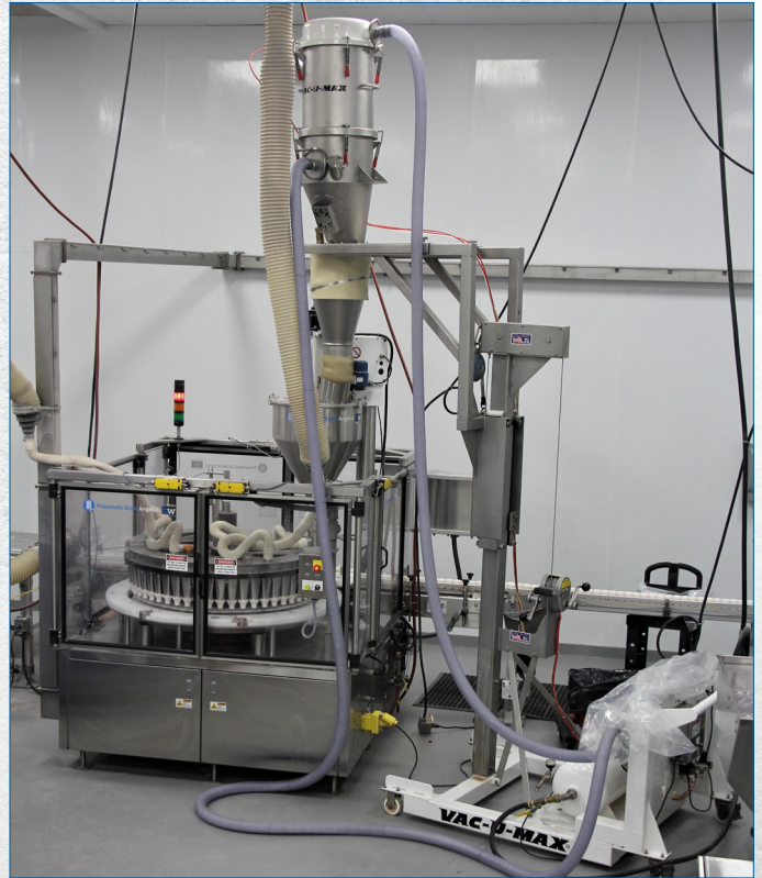
Mobile Vacuum Conveying System eliminates overhead conveyor installation, allows cleaning at floor level, and allows the system to be used in other packaging lines.
