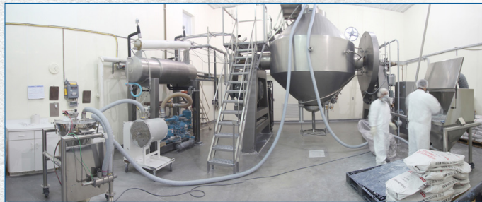
Ingredients are vacuum conveyed from floor-level and directly into tumble blenders without lifting, stair-climbing, and manual dumping of product.
