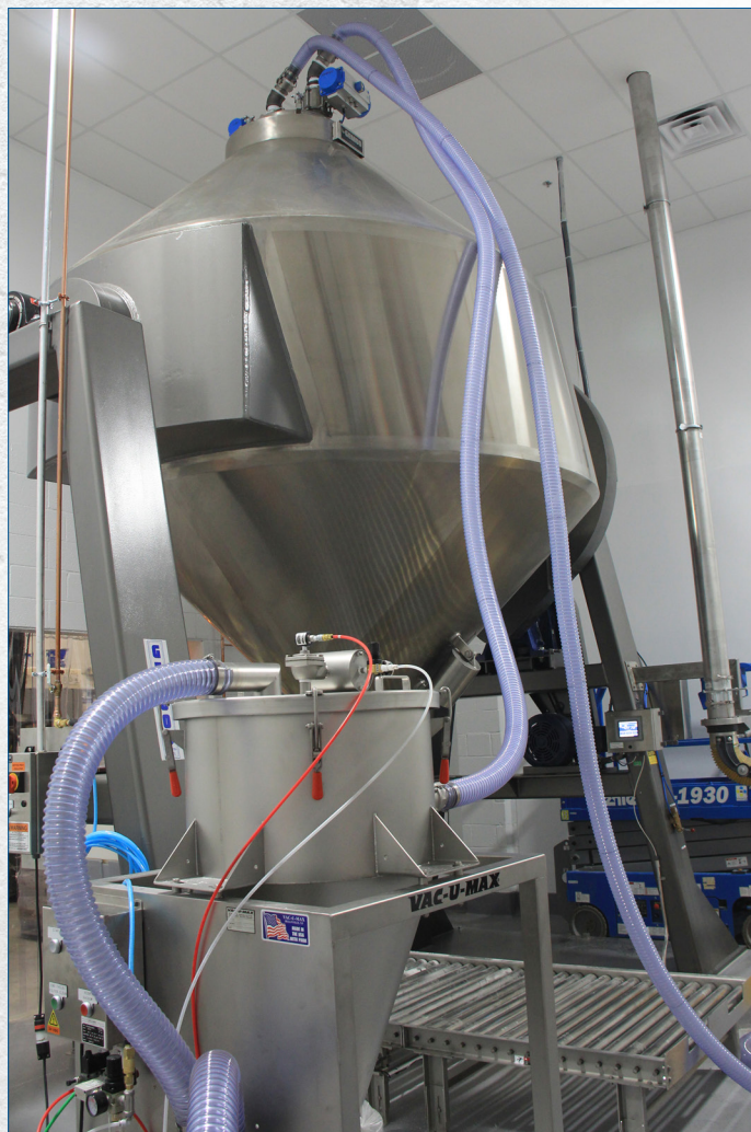
Direct-charge blender loading systems draw product from floor level to up, over, and into tumble blenders.
