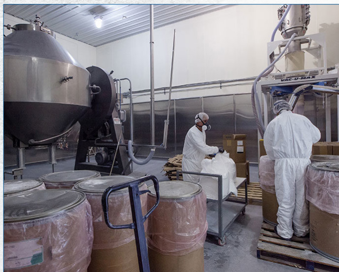
Product from floor level drums is easily vacuum conveyed into tumble blenders via wand, minimizing manual operation.
