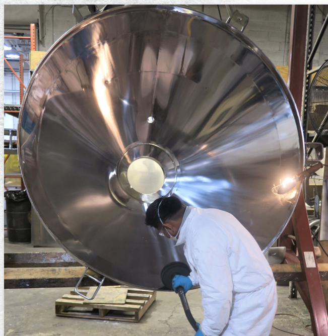
RA25 or lower finish and passivation are standard in the manufacture of sanitary components. rated for NEMA 4X.
