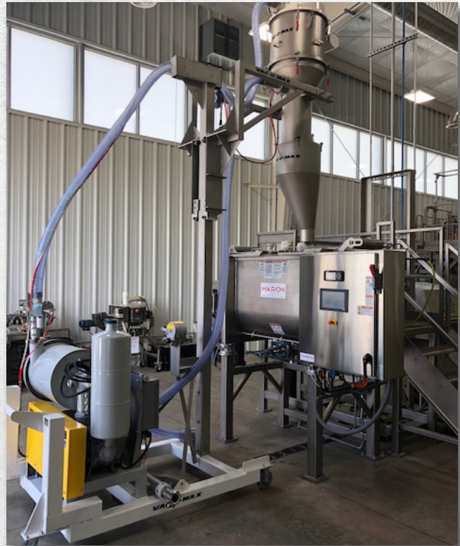
VAC-U-MAX Receiver conveys product to mixer, increasing productivity while greatly reducing sanitizing downtime.
